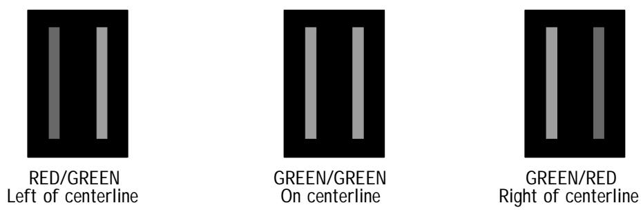
Figure 1. Centerline Guidance Light Unit
